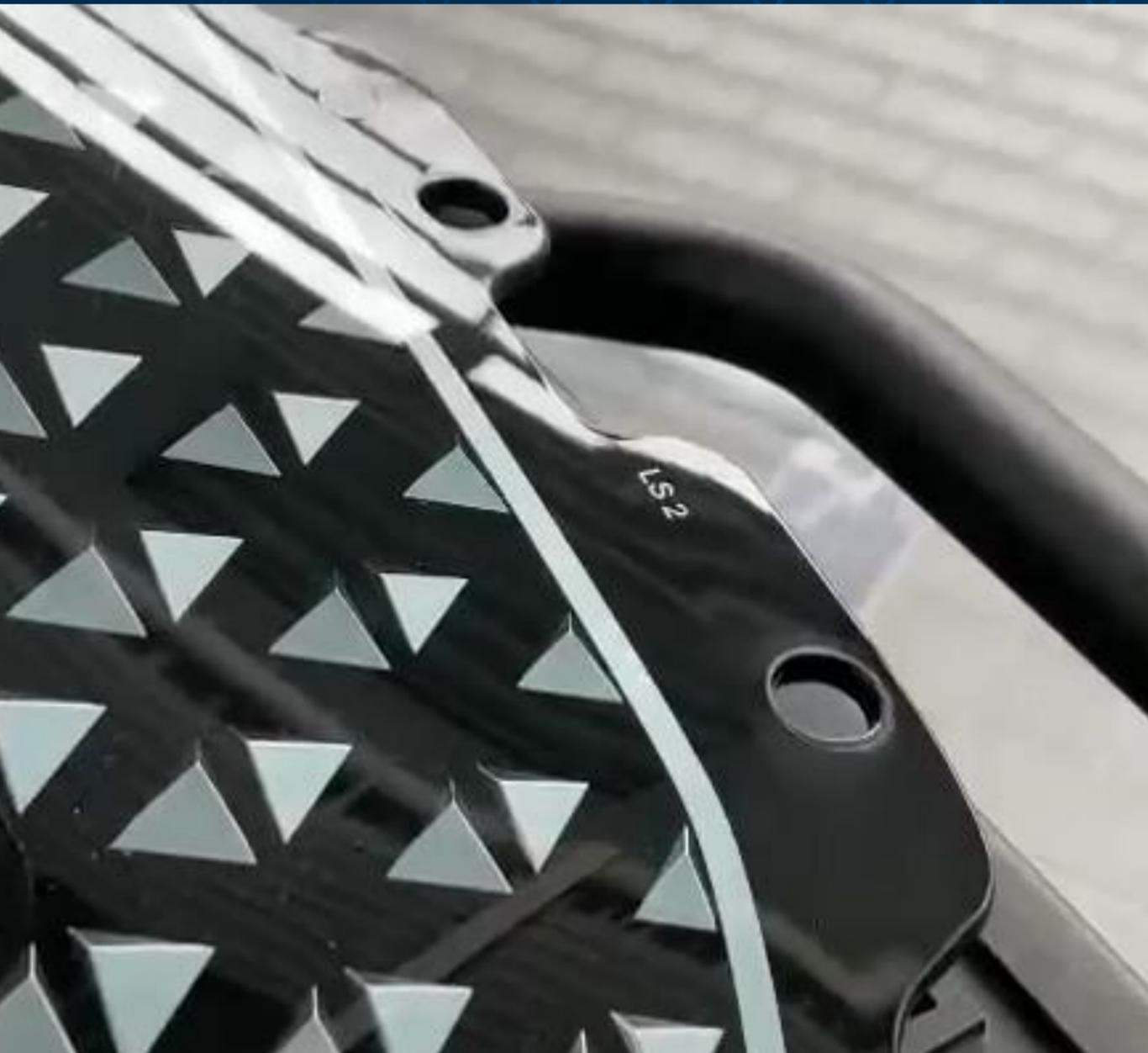
An additional polyurethane coating reduces the kidney grille's susceptibility to damage. The self-healing effect of its surface repairs minor scratches, for example – within 24 hours at room temperature or through a five-minute supply of warm air.
